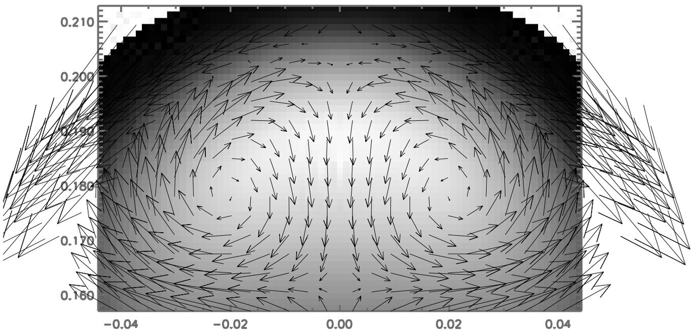
FIG. 3.—Close-up view of the tube interior showing the velocity vectors of the internal torsional oscillation at time  $t = 1.57$ . The arrows in the figure represent the relative velocity of the individual mass elements with respect to the tube apex.
