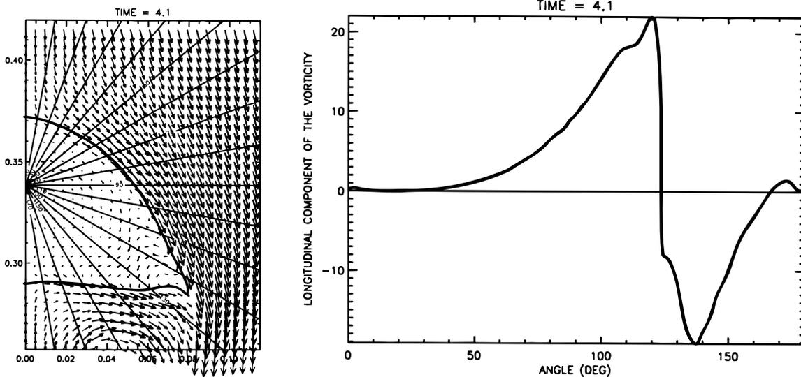
FIG. 10.—Profile of the longitudinal component of the vorticity (*right panel*) along the equipartition line drawn in the left panel for  $t = 3.8$ . The zero-crossing at about  $120^\circ$  corresponds to the transition from tube front to rear at the edge of the tube. The radial lines in the left panel are drawn at constant azimuthal angles.
