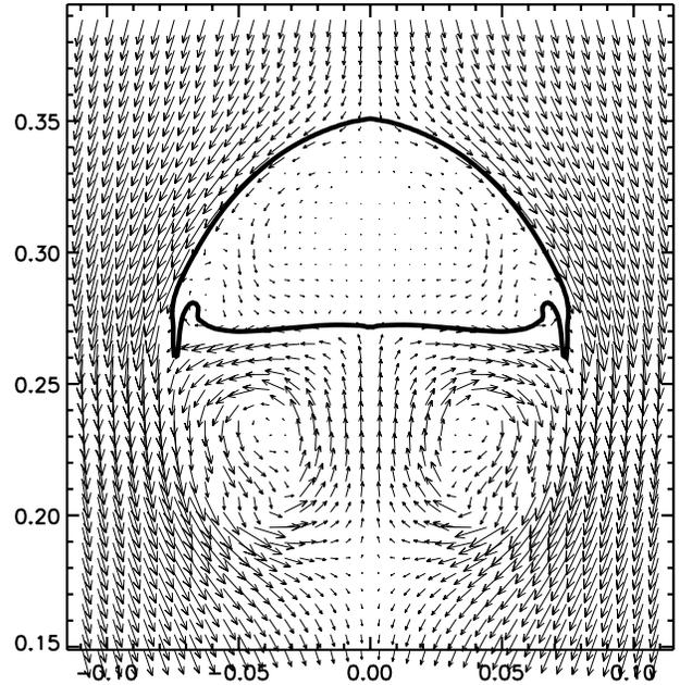
FIG. 5.—Equipartition line at  $t = 3.8$ , together with the flow field relative to the apex of the tube. The simple structure of the wake at this time is clearly visible. The envelope of the tube and the wake has a well-defined elliptical shape. This figure bears a strong resemblance to the experimental results of air bubbles rising in liquids (e.g., Collins 1965; also reproduced by Batchelor 1967, Plate 15).
