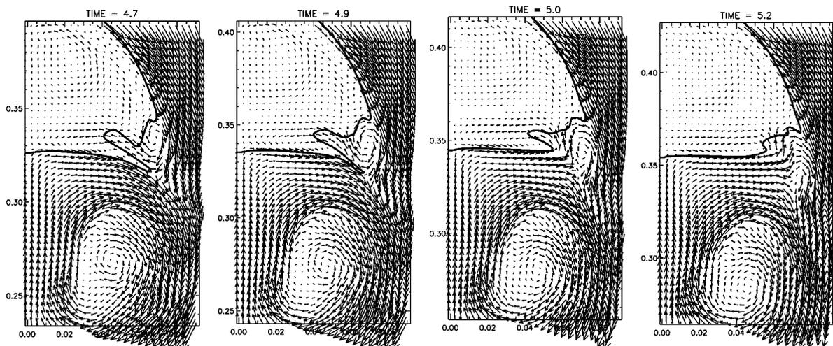
FIG. 13.—Formation and release of a secondary roll at the edge of the tube. The panels contain a time series showing the equipartition line and the relative flow field. The secondary roll is being released to the downflow; later on, it gets dragged all around the wake and noticeably perturbs the shape and velocity distribution. Note also the jumps in velocity inside the main roll of the wake, revealing the presence of vortex sheets that have been advected from the tube front.
